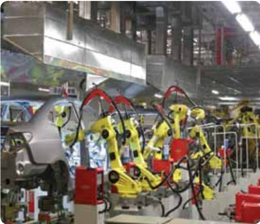
Arc welding robot
